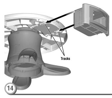
• Slide the tabs on the top of the oven into the track under the tabletop.
